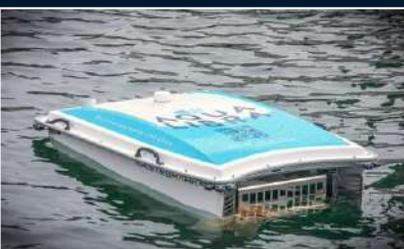
Powered by batteries, the WasteShark boasts an impressive range of up to five kilometres on a single charge, equivalent to eight to 10 hours of continuous cleaning. Every day, this environmental sentinel manages to extract approximately 500 kilograms of waste, equivalent to around 21,000 bottles.
